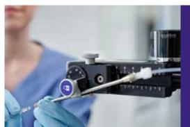
Swivel out function for easy capillary exchange. No need to remove the capillary holder from the manipulator for this purpose.
