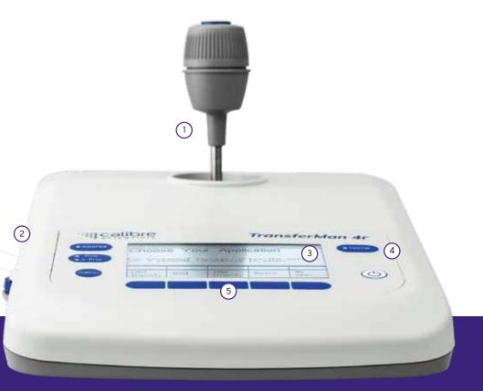
The unique DualSpeed<sup>™</sup> joystick combines precise and intuitive, direct movement with dynamic movement control for covering longer distances or speeding up sample processing. Furthermore, the dynamic movement mode can easily be switched off depending on the application need and personal preference.
