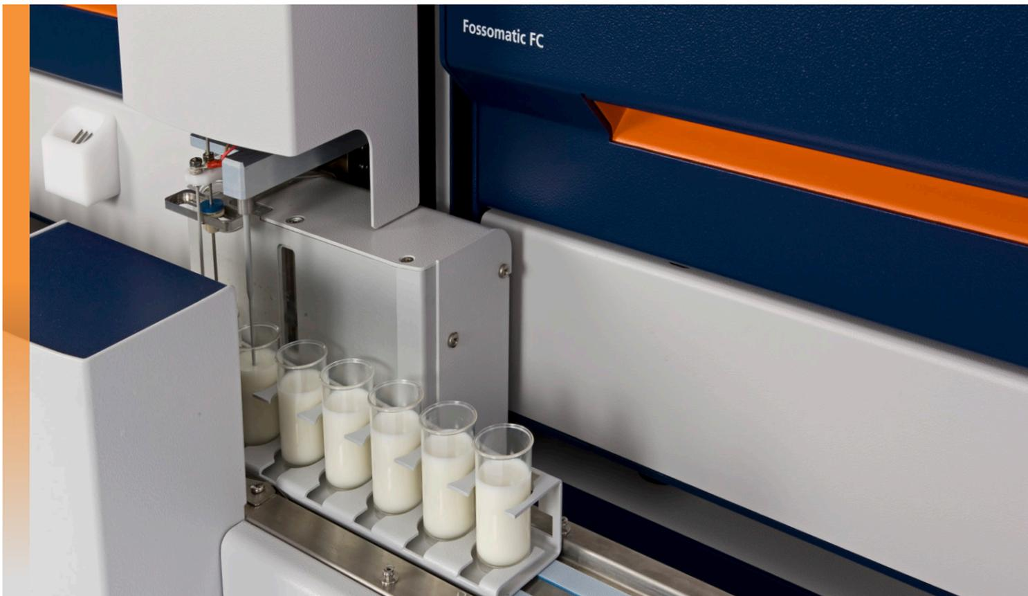
Fossomatic™ FC performs accurate milk analysis using somatic cell counting. It is a high capacity analyser (up to 600 samples per hour) that meets the demands of farmers in need of fast and reliable payment and Dairy Herd Improvement (DHI) results. Fossomatic™ FC is based on flow cytometry technology that counts somatic cells in compliance with ISO/IDF and FDA/NCIMS standards.
