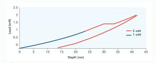
Low load nanoindentation curves on single crystal sapphire. Contact is completely elastic until a pop-in at 1.5 mN.
