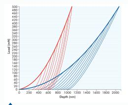
Consistency of NanoTest results shown by loading curve superimposition in repeat nanoindentations at different positions to peak loads of 100-500 mN. Sets of 10 load/unload indentations obtained over a wide depth range. The overlapping loading curves demonstrate excellent consistency. Each load/unload curve produces hardness and modulus values corresponding to its particular depth of indentation.
