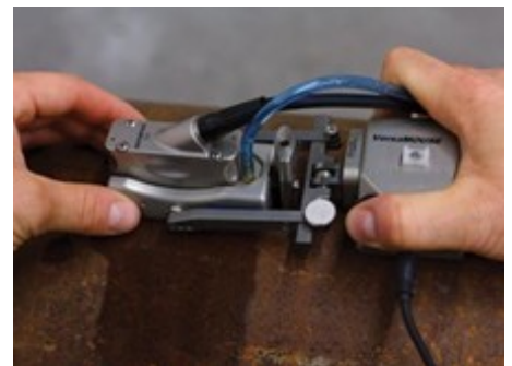
VersaMOUSE and RexoFORM scanners for corrosion inspection.
