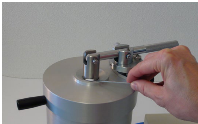
Introducing the powder in the Nebula Particle Dispenser for creation of a uniform monolayer.
